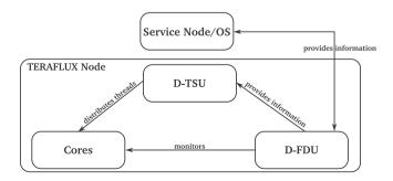
Fig. 9. Interaction between TERAFLUX Nodes, Service Node, Distributed-TSU (D-TSU) and Distributed FDU (D-FDU).
