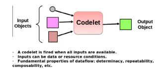
**Fig. 12.** The Codelet: a Fine-Grain Piece of Computation. A codelet is fired when all inputs are available. Inputs can be data (square inputs) or resource conditions (gray circle).
