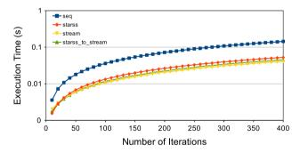
**Fig. 7.** Gauss-Seidel experiment for a 256  $\times$  256 matrix, with 64  $\times$  64 blocks. The benchmark was run on 12 cores. Four versions executed: OpenStream ('stream'); StarSs ('starss'); an OpenStream-StarSs combination ('starss\_to\_stream'); and a sequential version ('seq'), used as the baseline.
