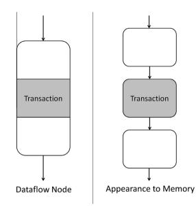
**Fig. 4.** On the left a node in the dataflow graph containing a transaction, on the right how this can be viewed as three nodes by the memory system.
