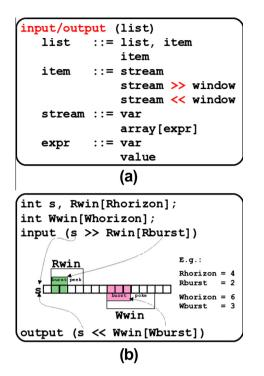
Fig. 6. Syntax for input and output clauses (a) and illustration of stream access through windows (b).
