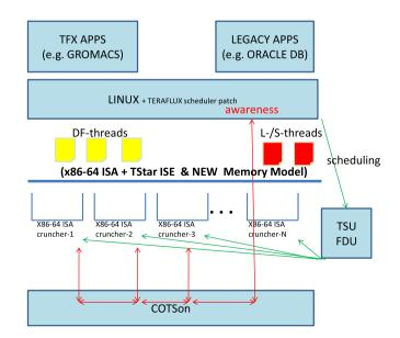
**Fig. 11.** Overall picture of the "simulator illusion". A number n of VCPUs can be used as "workers" or "x86\_64 crunchers" or "Auxiliary Cores" or "Service Cores"; a generic *k*th VCPU can be used as service core. L- and S-threads represent Legacy and System Threads, that our system is able to execute.
