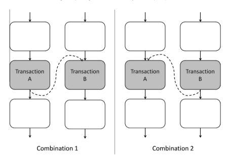
Fig. 5. The two possible formulations of a section of the dataflow graph containing two conflicting transactions. The dashed data dependency will be inserted and enforced at runtime by the transactional memory system, making the relationship between transactions part of the dataflow graph.
