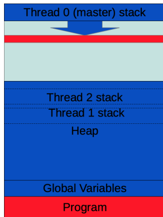
Figure: Multithreaded Process: Memory
