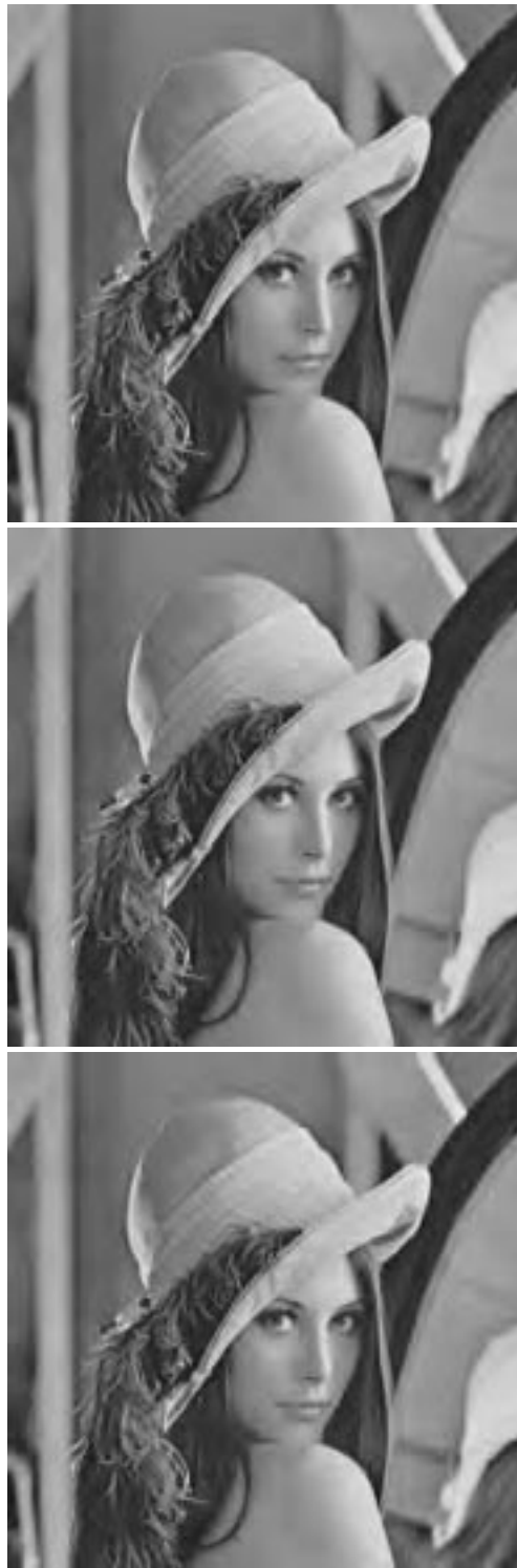
Figure 6: Lena at 0.1 bpp, from top to bottom: 9/7-tap biorthogonal (30.23 dB PSNR), 8-tap multiwavelet (balancing order 2, 29.78 dB), 12-tap multiwavelet (balancing order 3, 29.83 dB)
