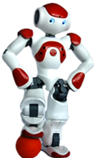
Fig. 1. The robotic platform used in the present system: Nao from Aldebaran Robotics.
